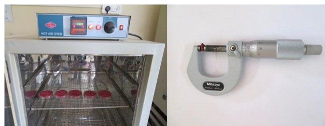
Fig 1: Determination of moisture content and seed size of cotton
