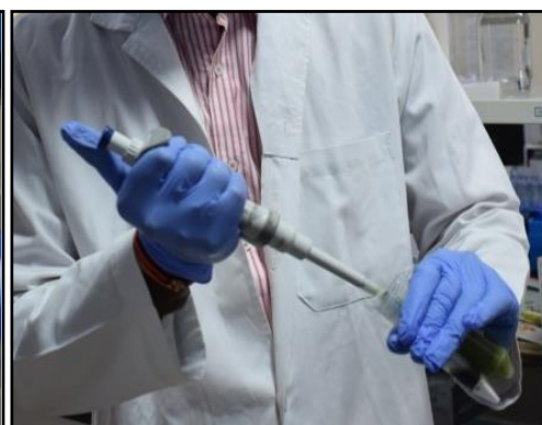
Transfer of 7 ml extract to 15ml centrifuge tube containing 25mg PSA and 150mg \text{MgSO}_4
