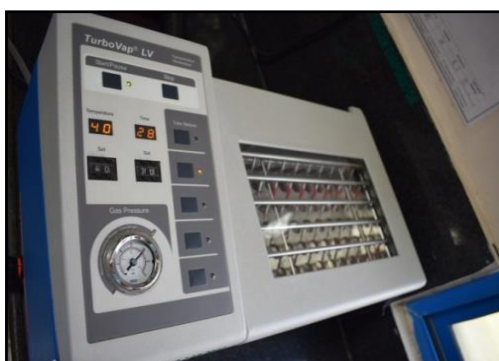
Homogenization, high volume centrifugation, evaporating to dryness using nitrogen concentrator
