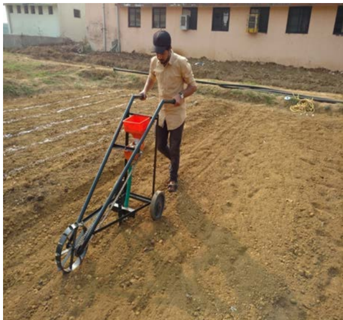
Fig 2: Developed vegetable planter
