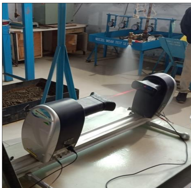
Fig 1: Malvern Spraytec system setup for nozzle test
