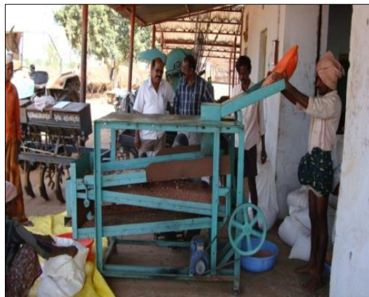
Fig 3: Groundnut kernel grader
