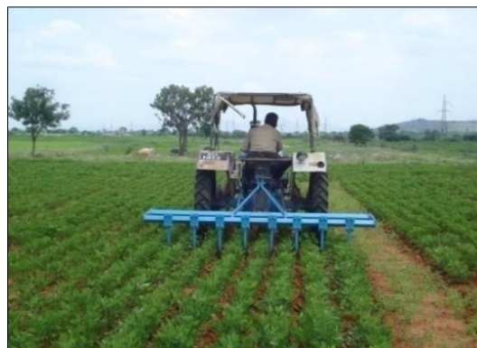
Fig 7: Ananta tractor drawn inter-cultivation implement
