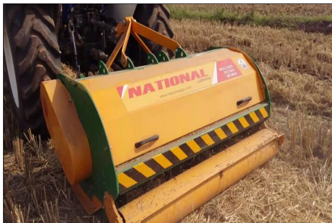
Fig 4: Mulcher Paddy straw and stubbles cut and spread in the surface
