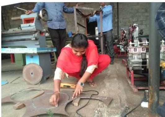
Fig 1: Marking for casing
