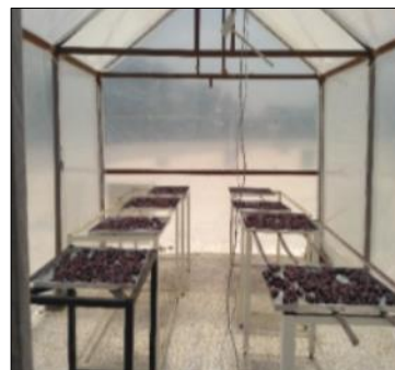
Fig 4: Trays loaded with date palm fruits inside the greenhouse dryer
