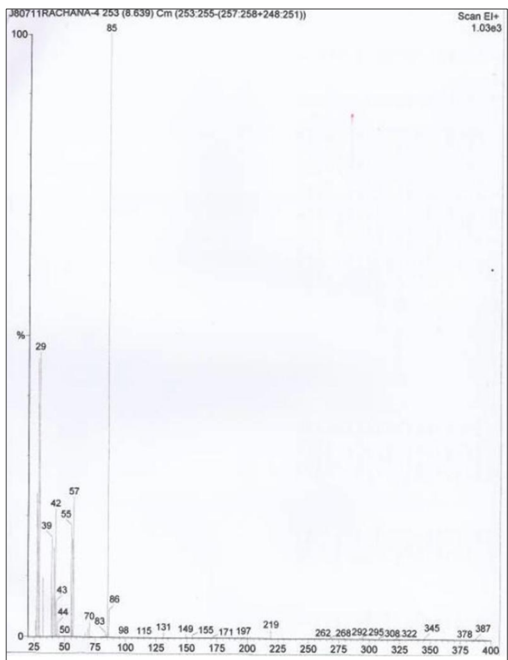
Fig 2: Mass spectra of peak no. 3 (RT-8.694) of chromatogram
