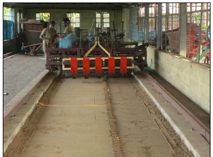
Plate 3: Loading car assembly with pulse planter
