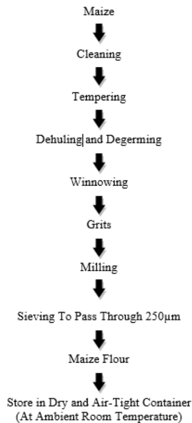
Fig 2: Flow diagrams for the preparation of maize-flour
