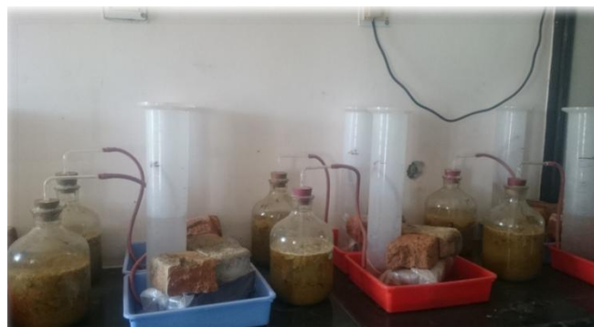
Fig 1: Experimental set up of a laboratory scale anaerobic tubular digester.
