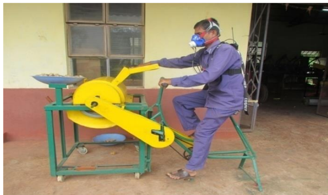
Fig 2: VO 2max measurement while operating pedal operated arecanut dehusker
