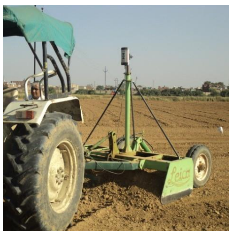
Fig 3: Shaping of field \pm 2 cm at 100m by laser-assist precision land leveller
