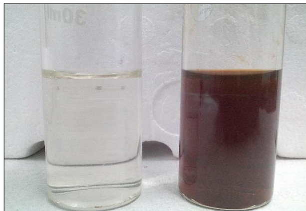
Photo 2: Reaction mixture (10 ml of AgNO 3 and 1ml of soybean seed extract) before (left) and after (right) exposing to sunlight
