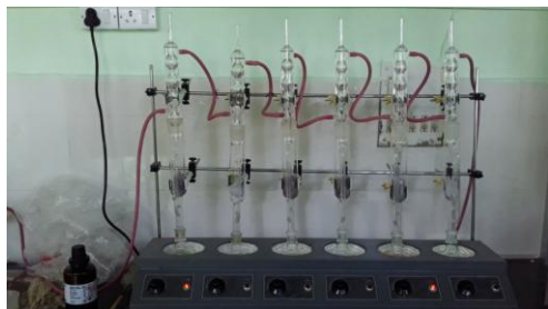
Fig 7: Soxhlet apparatus setup used during oil extraction
