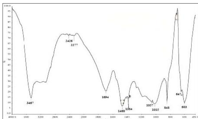
Fig 3: FT-IR spectrum of S. asperum mediated synthesized silver nanoparticles
